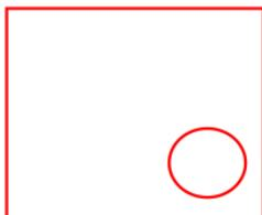
The circle rests inside the rectangle. The geometries can be sorted and cutting will start with the circle.
