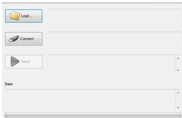
Choose Firmware File. Connect to Engraver (machine must be started with open top cover, or referencing has been finished) Press Send to process Firmware Update.
